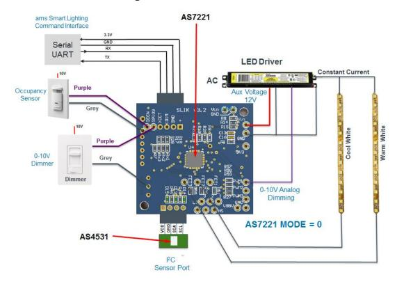
As shown above, a Color Tuning AS7221 SLIK adds Daylighting with a simple inclusion of an AS4531 via I<sup>2</sup>C:
